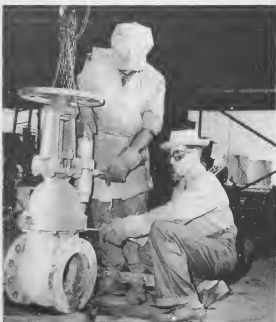
George Wellington (standing) and George Wellington (pará) y Antón Antón Riddersstaal break open a two-inch valve for inspection purposes.
